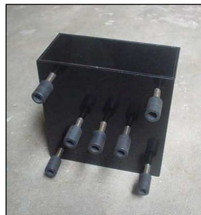
Fig. 8. Portable spring loaded electrode holder for lungs ventilation mapping using FIM.
