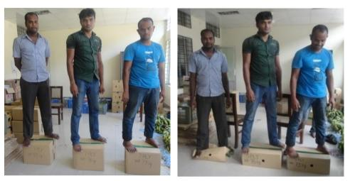
Fig. 4. Measuring the static load bearing capacity of the carton.
