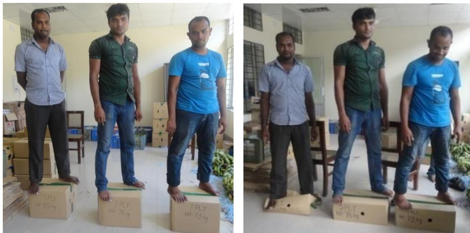
**Fig. 4. Measuring the static load bearing capacity of the carton.**
