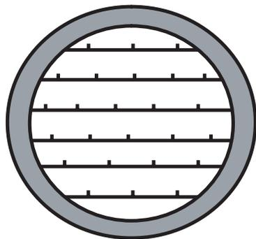
**Fig.-2:** Figure of an integrating eye-piece with 25 points which was used to measure the interstitial tissue of the kidney
