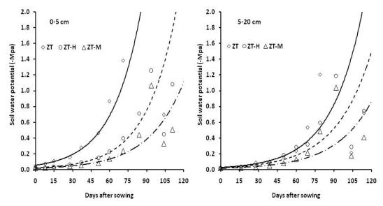
Fig. 5. Soil drying out pattern under zero tillage (ZT) with stubble height (ZT-H) and with mulch (ZT-M)
