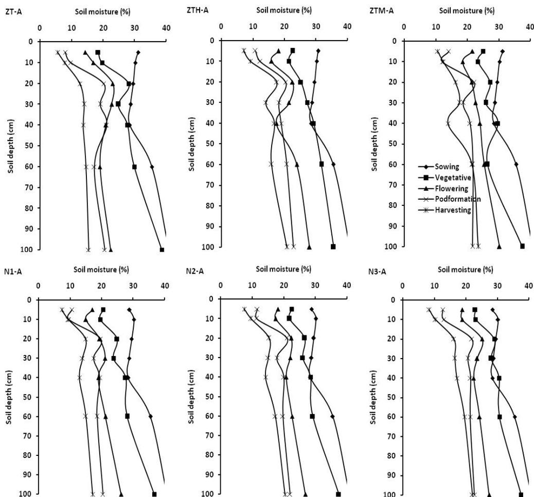
Fig. 1. Distribution of moisture within soil profile at critical growth periods under different nutrient and residue management practices (pooled data of three years with var. Asha)
