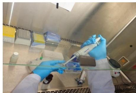
**Figure 4. Master mix preparation in BSL-2 cabinet.**
