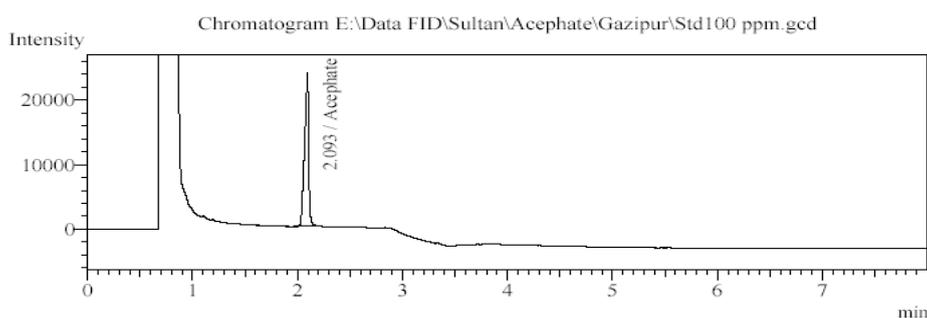
**Figure 3. Chromatogram of acephate standard solution.**
