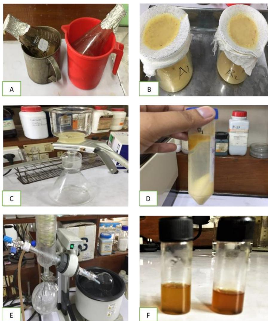
**Figure 9.** Photograph showing recovery of organic acid from fermented broth while thawing after freezing (A), vacuum filtration (B, C), centrifugation (D), and rotary evaporation (E) and concentrated lactic acid after evaporation (F).
