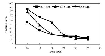
Fig.2: Effect of radiation dose and concentration of CMC on Swelling Ratio of 5%Acryl Amide/CMCblend hydrogel in deionized water
