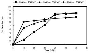
Fig. 1: Effect of radiation dose and concentration of CMC on gel fraction of Acrylamide /CMC blend hydrogels
