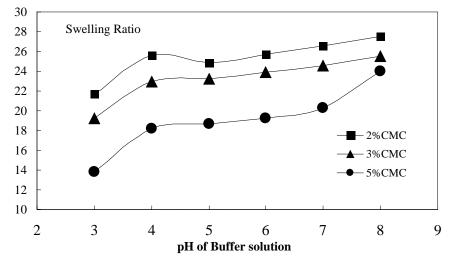
Fig. 4. Effect of concentration of CMC on swelling ratio of Am/CMC blend hydrogel in buffer solution at 25kGy [standing time 48h]
