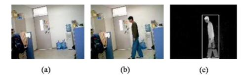
Fig. 1. Extraction of region of interest (ROI). (a) Background (b) Human in foreground and (c) After background subtraction.
