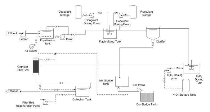
Figure 1: PFD of physico-chemical treatment of paper mill effluent (raw material: imported pulp/recycled paper)
