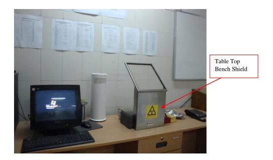
Figure 1: A commercial table top bench shield
