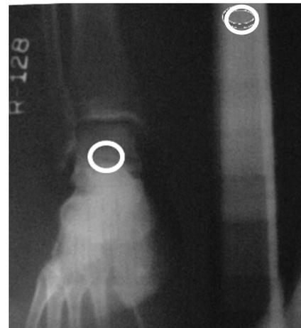
Fig.9: X-ray image of ankle of subject 1 beside that of aluminium strips. The circled areas on both the ankle and the aluminium strip image had equal density values.
